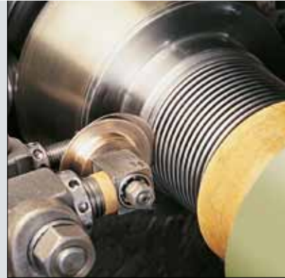
SAMSON produces its bellows from corrosion-resistant materials
