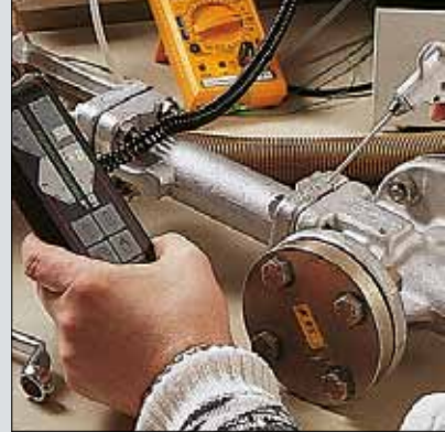
Helium leak testing according to the sniff or vacuum method
